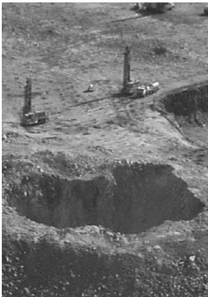
Figure 3: Voids from old workings at a West Australian Gold Mine.
