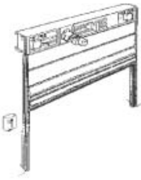
Figure 9: Schematic and photographic views of a roller door regulator.
