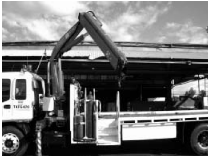
NO GO ZONE PREVENTS BOOM FROM SLEWING INTO OPERATORS ZONE
