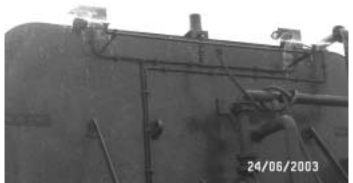
Image 2: Nozzles are activated on rear spray control circuit.
