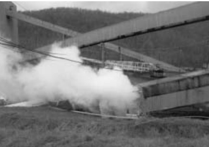
Figure 4: Seal after blow out.
