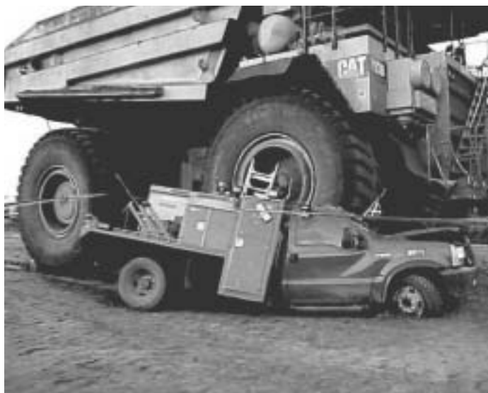
Figure 9: Damage inflicted on a light vehicle when run over by a haul truck.
