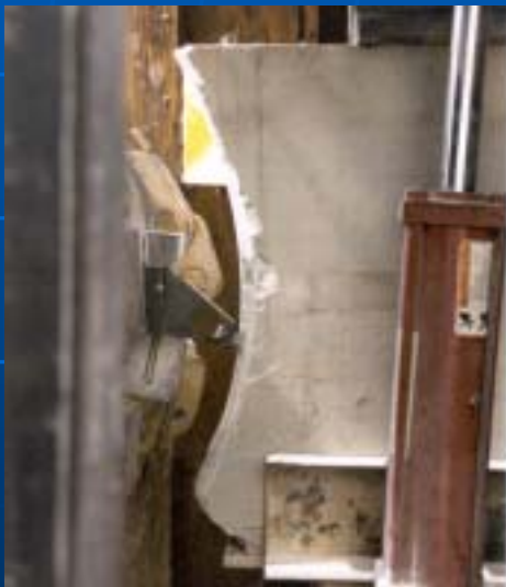
Miner bit cutting into sandstone block
