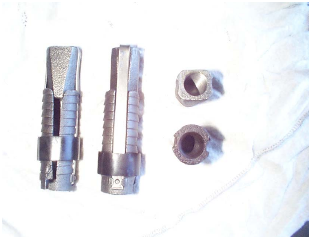
Figure 5: Modified expansion shell anchor for use with the PAG bolt. Note the differences between the trimmed and standard barrel.
