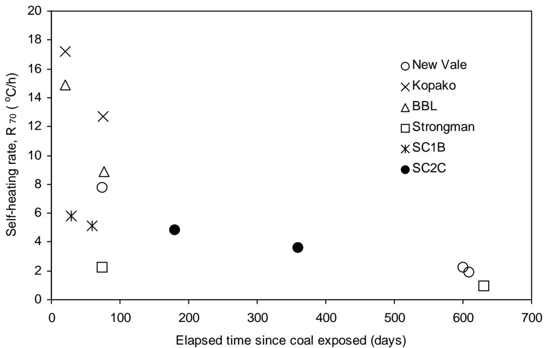
Fig. 5. Self-heating rates of repeat tests on stored New Zealand and Australian coals.
