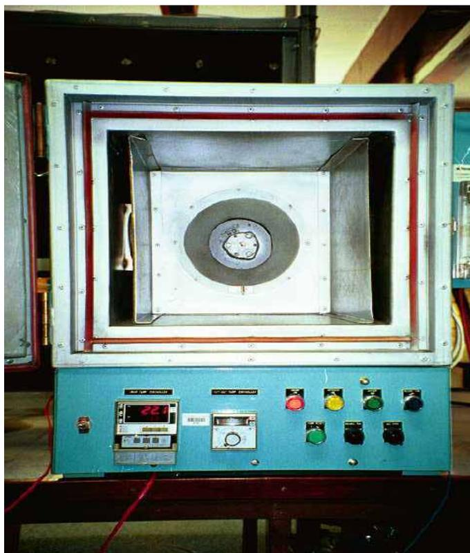
Fig. 1. Interior view of the adiabatic oven.
