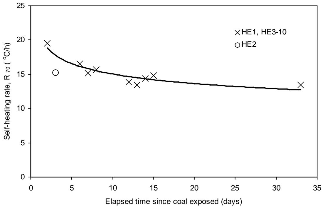
Fig. 4. Self-heating rates of repeat tests on Huntly East subbituminous coal.
