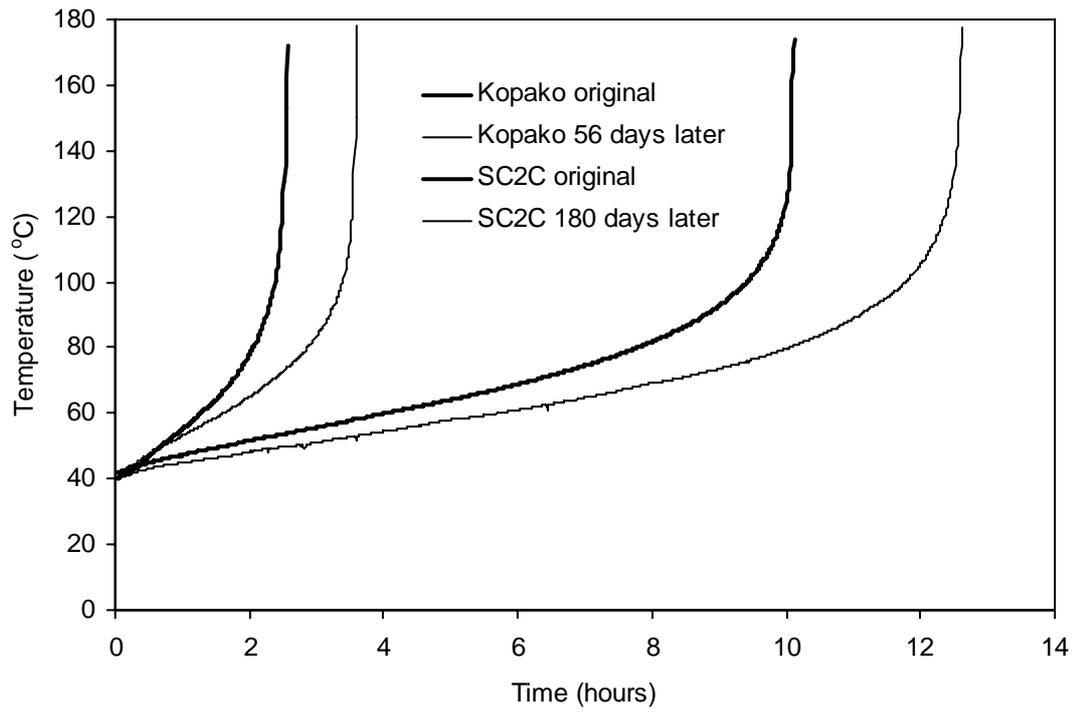
Fig. 3. Repeat self-heating rate profiles for Kopako (61/814) and Dunn Creek (SC2C).
