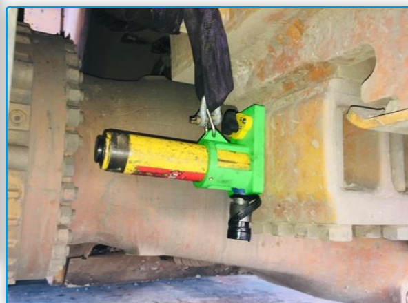
Photo 2 – Cylinder in place with new adaptor & lanyard
