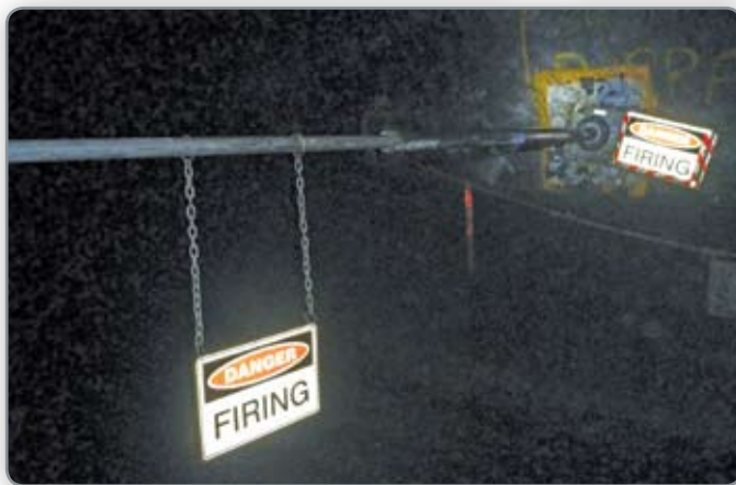
Photo 4: Telescopic Barricade in "opened position"
