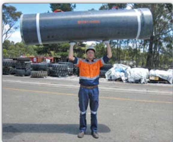
Photo 1: Carbon fibre ventilation tube weighing 9kg
