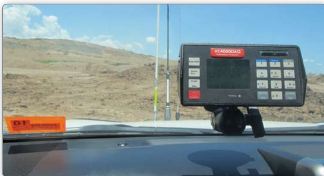
Road friction test Instrument mounted in test vehicle.
