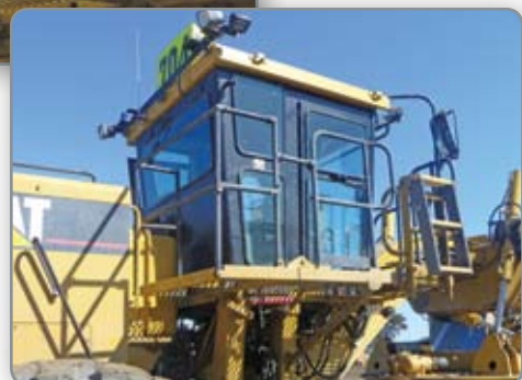
Picture 3 Access platform in the deployed position.
