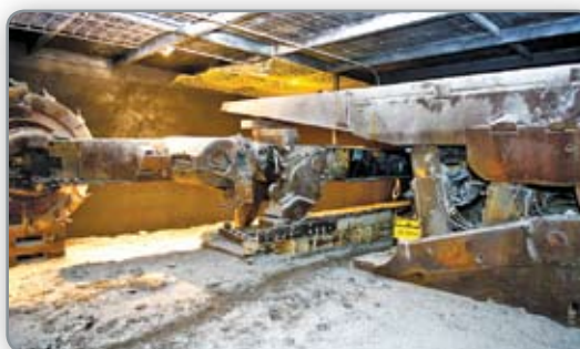
Longwall chocks and shearer arm in Myne Start training complex
