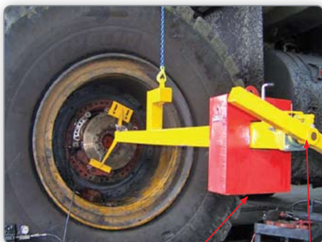
Two Position Counterweight (155kg)
