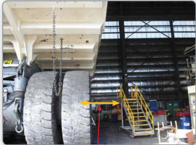
Coal Tray width did not allow using the lifting crane.
