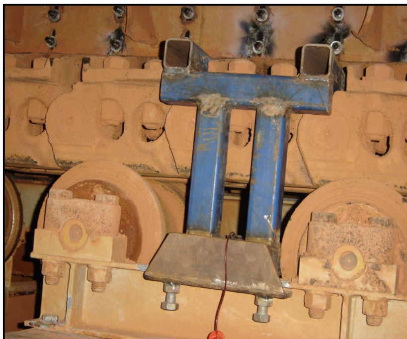
Figure 1: The locking tool attached to the apron feeder assembly.
